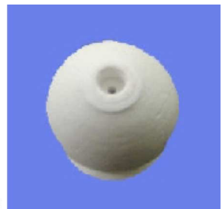
Fig. 13. CAD project of ceramic nozzle (a). Ceramic nozzle produced with STL (b).
